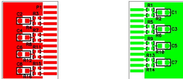
Figure 4.3 Example termination pads
