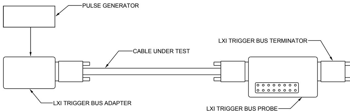
**Figure C.1 Wired pairing test setup**
