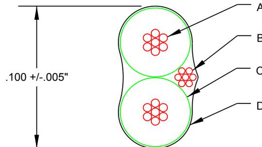
**Figure 2.1 Single Twisted Pair Assembly**
