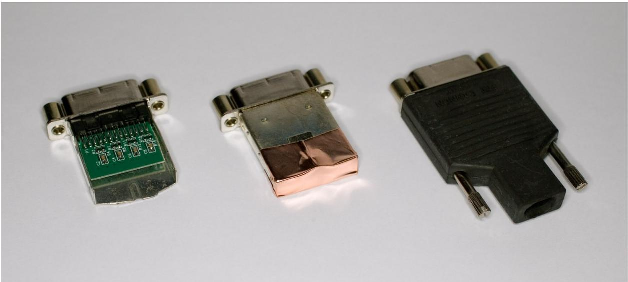
**Figure 4.1 Example LXI Wired Trigger Bus Terminators**
