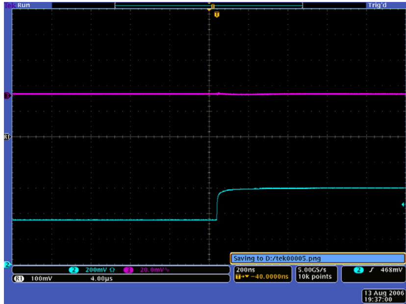
Figure 3.5 – 20 meter cable displaying no cross-talk
